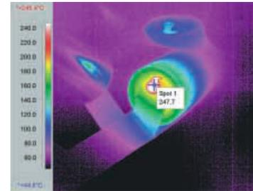
A series of failing idlers on the coal handling line were located by using a Thermographic system.
