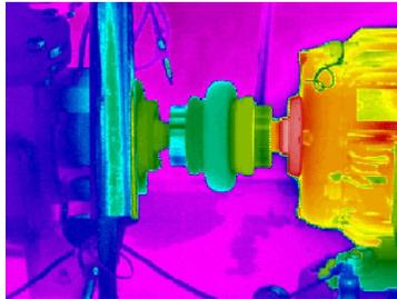
Thermography can easily identify all types of impending drive problems during plant operation.
